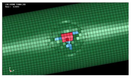
LS-DYNA result of explosive rupture of railcar (source: Florida A&M University)
