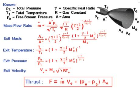
Solid rocket motor thrust equations (source: NASA)
