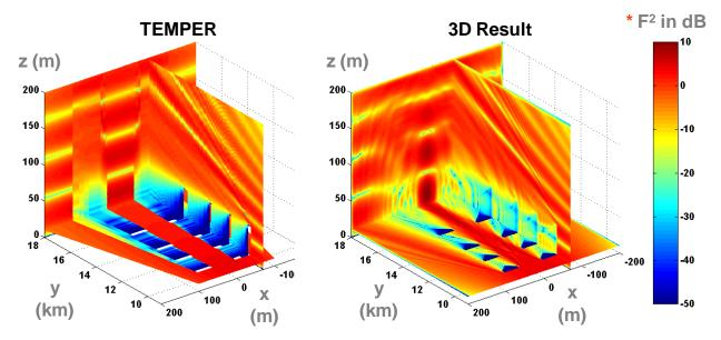
Propagation factor "F"  $\equiv$  | E / E<sub>o</sub>| where E<sub>o</sub> is free-space field
