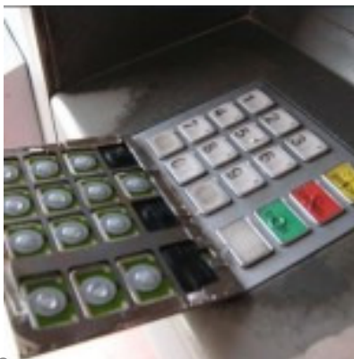
Skimming Pad on top of legitimate Pin Pad
