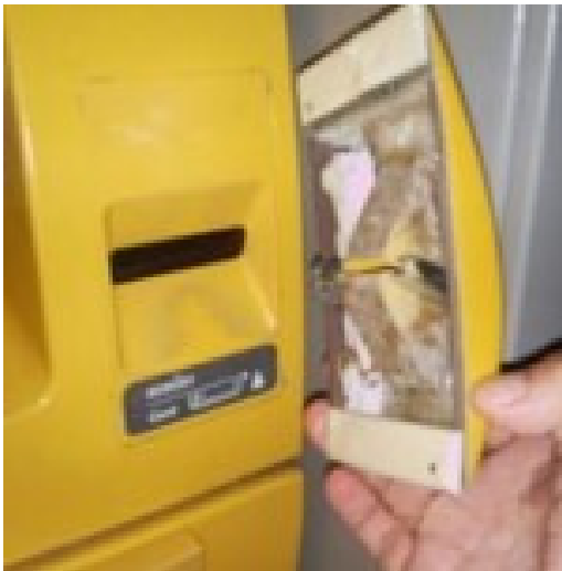
Skimming device removed from ATM
