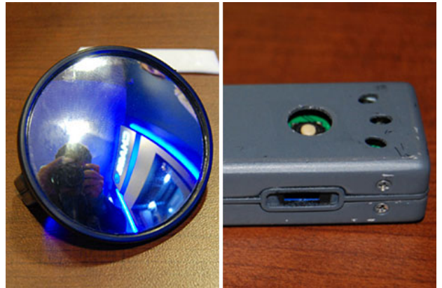
Skimming device and mirror removed from ATM
